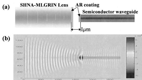
Fig. 4. Focusing in a SHNA MLGRIN lens from the optical fiber mode to a III-V waveguide with an air gap and an antireflection (AR) coating: (a) structure, (b) FDTD simulated TE-light  $E$ -field pattern ( $V \times H=13 \mu\text{m} \times 28 \mu\text{m}$ ).
