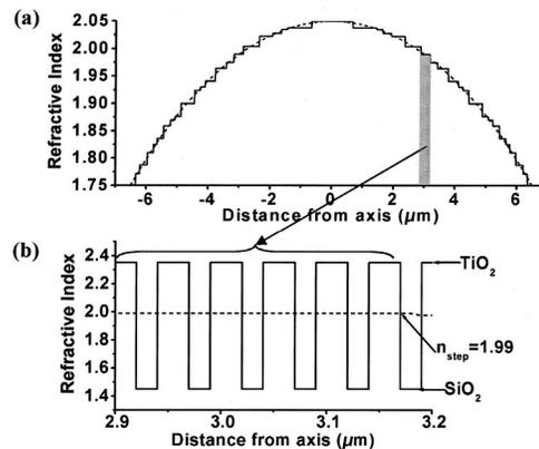
Fig. 1. (a) Parabolic refractive-index profile (dashed curve) of a  $13\text{-}\mu\text{m}$ -thick GRIN lens and the approximate step refractive-index profile of a SHNA MLGRIN lens (solid curve). (b)  $\text{TiO}_2$  and  $\text{SiO}_2$  layers (solid curve) used to approximate a certain step refractive index (dashed line).
