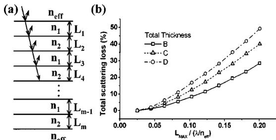
Fig. 2. (a) Layer structure used in estimation of scattering loss by the transfer matrix method. (b) Total scattering loss calculated by the transfer matrix method for three total structure thicknesses: 3  $\mu\text{m}$  (B, solid curve), 5  $\mu\text{m}$  (C, dashed curve), and 7  $\mu\text{m}$  (D, dashed-dotted curve).
