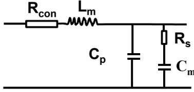
**Fig. 2. Equivalent circuit of traveling-wave EO modulator.**
