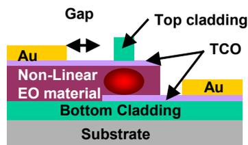
**Fig. 1. Structure of TCO modulator with side injection configuration.**
