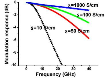
**Fig. 3. Dependence of modulation bandwidth on conductivity of TCO.**
