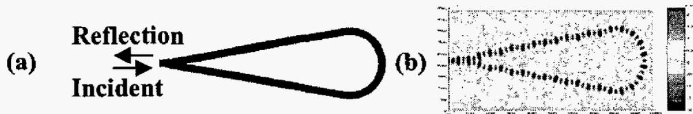
Fig. 1. (a) High reflection loop mirror with 20 degree angle and  $3\mu\text{m}$  diameter waveguide loop, (b) FDTD pattern of the electrical field when launching in CW wave at wavelength  $1.55\mu\text{m}$ .
