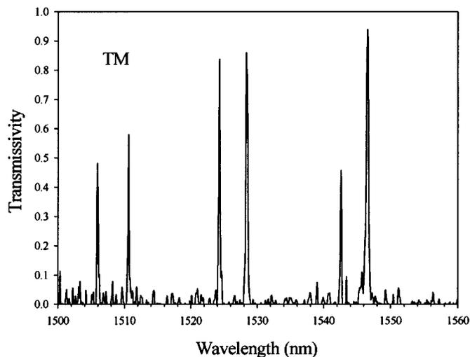
Fig. 3. Measured transmissivity as the function of wavelength of a 10- $\mu\text{m}$ -diameter BCB bonded microdisk resonator for the TM case.
