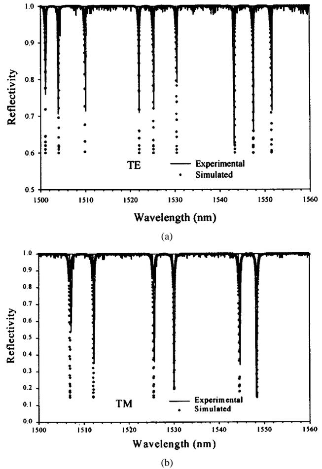
Fig. 2. Reflectivity as the function of wavelength of a 10- $\mu\text{m}$ -diameter BCB bonded microdisk resonator with coupling waveguide. —Experimental ... Simulated (a) TE and (b) TM.
