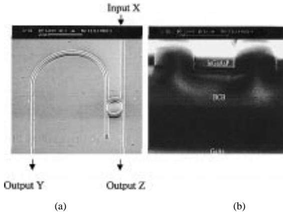
Fig. 1. (a) Scanning electron microscope (SEM) image of a 10- $\mu\text{m}$ -diameter BCB-bonded microdisk resonator with coupling waveguide. (b) Cross section of a BCB bonded waveguide.
