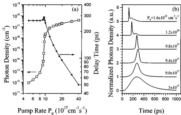
FIG. 3. Calculated results when the pump pulse width is 400 ps. (a) The maximum photon density and delay time as a function of the pump rate. (b) The temporal evolution of the photon density at several pump rates as indicated.
