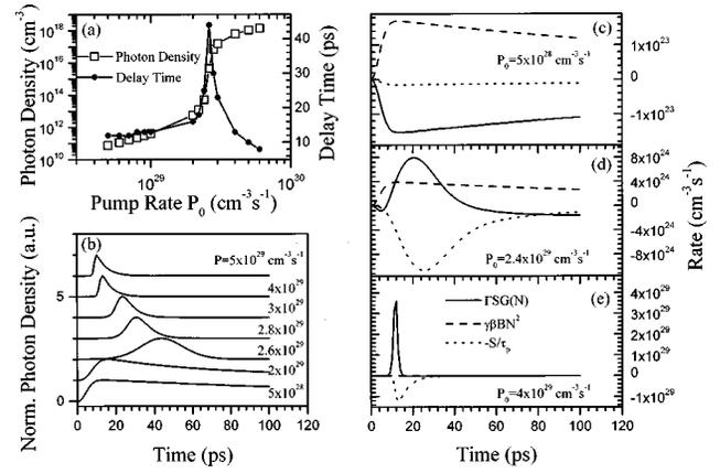
FIG. 2. Calculated results when the pump pulse width is  $10 \text{ ps}$ . (a) The maximum photon density and the delay time vs the pump rate. (b) The temporal evolution of the photon density at several pump rates as indicated. (c)–(e) The time-resolved traces of  $\Gamma SG(N)$  (solid line),  $\gamma \beta BN^2$  (dashed line), and  $-S/\tau_p$  (dotted line) at several pump rates as indicated.
