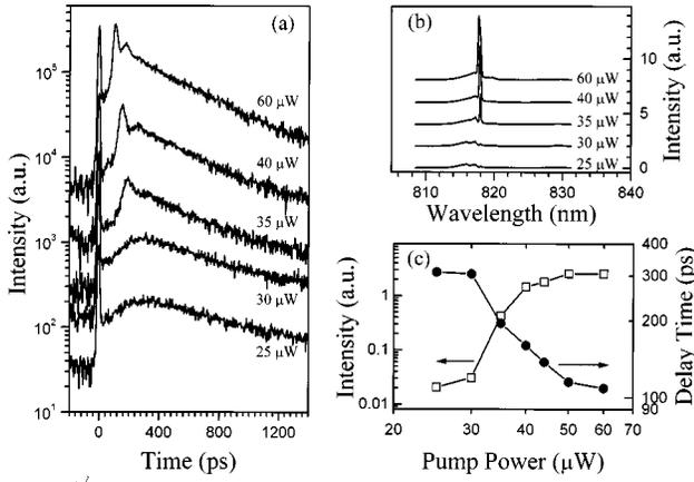
FIG. 1. (a) Experimentally observed temporal evolution of microdisk emission. (b) Time-integrated emission spectra. The incident pump powers are marked next to the curves, which are shifted vertically for clarity. (c) The integrated emission intensity and the delay time as a function of the incident pump power.
