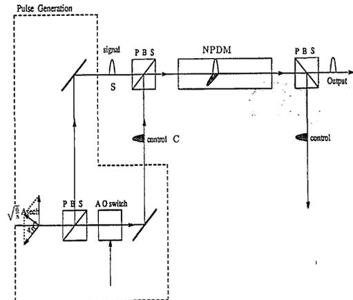
Fig. 1. Schematic of light-by-light switching based on the transmission of coupled gap solitons. AO, acousto-optical.
