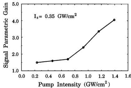
Fig. 5. Normalized degenerate OPA gain of the input signal as a function of pump intensity inside the AlGaAs waveguide.
