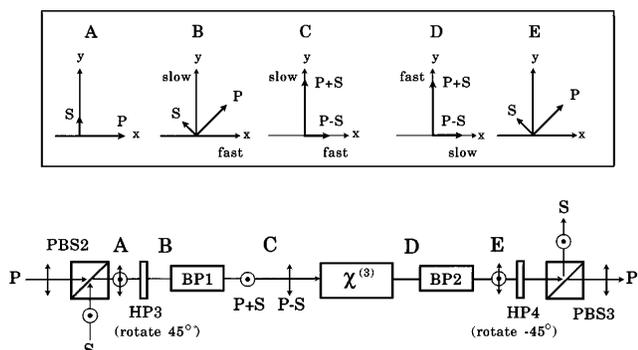
Fig. 2. Novel pulse-delayed DOPA scheme.
