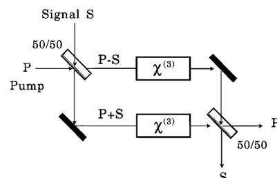
Fig. 1. NMZI scheme for a  $\chi^{(3)}$ -based degenerate OPA.
