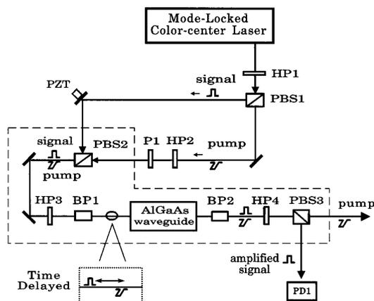
Fig. 3. Experimental setup to demonstrate the pulse-delayed DOPA, using AlGaAs waveguides.
