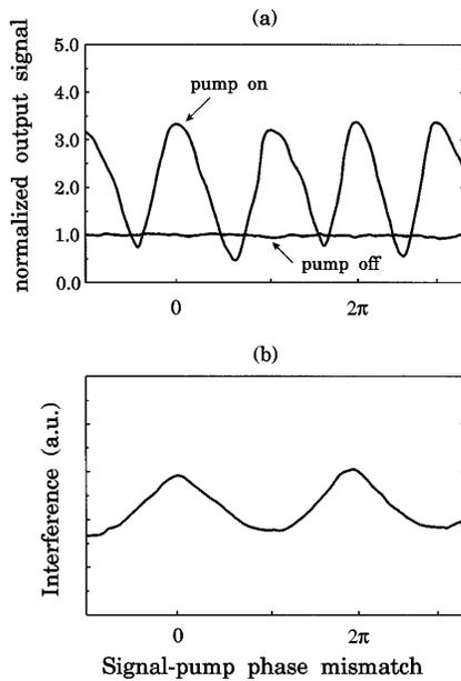
Fig. 4. (a) Normalized output signal for the cases when the pump is on and off:  $I_p = 1.16 \text{ GW/cm}^2$  and  $I_s = 0.35 \text{ GW/cm}^2$ ; (b) interference between pump and signal as a function of the pump–signal phase mismatch.
