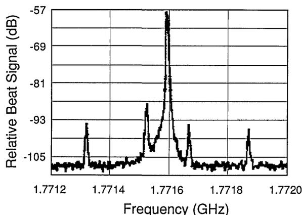
Fig. 2. Spectrum of the beat signal between the Raman-laser beam and the pump beam in the vicinity of 1.772 GHz. The horizontal scale is 200 kHz per division, and the vertical scale is 6 dB per division. The resolution bandwidth of the spectrum analyzer was 3 kHz, and the sweep time was 6.7 s.
