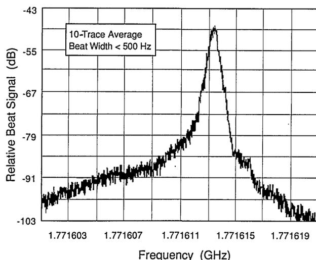
Fig. 3. Expanded view of the center peak in Fig. 2. The horizontal frequency scale is 2 kHz per division, and the vertical scale is 6 dB per division. The resolution bandwidth of the spectrum analyzer was 215 Hz, and the sweep time was 2.8 s. The trace was video averaged 10 times. The FWHM bandwidth of this beat is 440 Hz.
