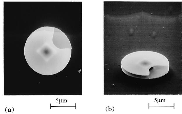
FIG. 3. Scanning electron microscope images of a fabricated double-disk microdisk laser with  $10 \mu\text{m}$  in diameter. (a) top view; (b) side view.
