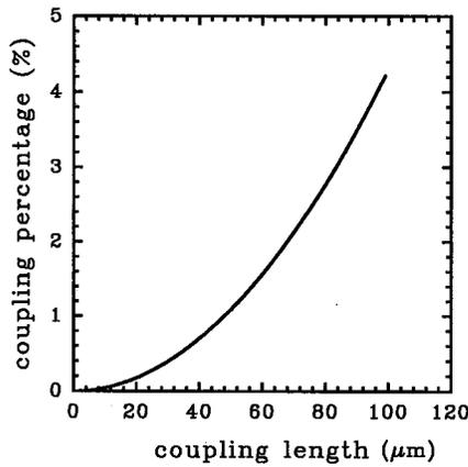
FIG. 2. The calculated coupling efficiency per roundtrip length of a two-disk structure vs the coupling length, which is approximately the circumference of the disk structure. The separation between the two disks is assumed to be  $0.65 \mu\text{m}$ .
