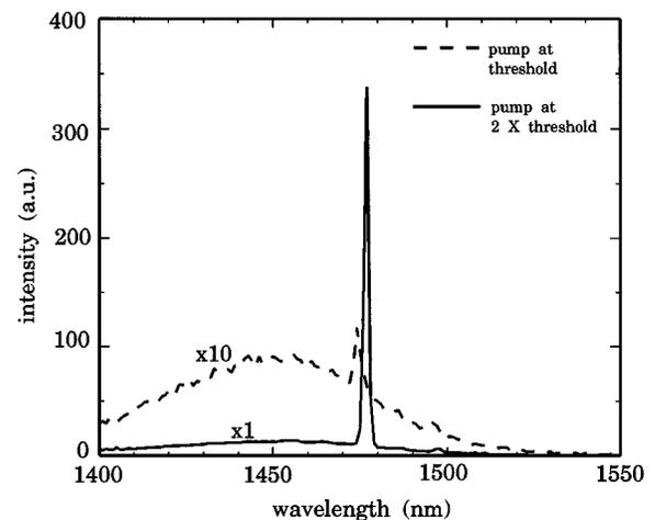
FIG. 4. Measured spectra of the  $10\text{-}\mu\text{m}$ -diam double-disk microdisk at  $85 \text{ K}$ . Excitation is by a Nd:YAG laser at the wavelength of  $1064 \text{ nm}$ . The solid curve is for the case where the pump power is above threshold and the dashed curve is for the case where the pump power is at threshold. The resolution of the spectrometer is  $1 \text{ nm}$ .
