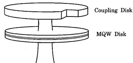
FIG. 1. Schematic of the double-disk structure of the InGaAs/InGaAsP microdisk laser in our experiments. The top disk, basically a passive guiding disk, receives lasing light from the bottom MQW disk structure through resonant waveguide coupling. The opening on the top guiding disk provides a leaking source and directs the lasing light out from the double-disk structure.
