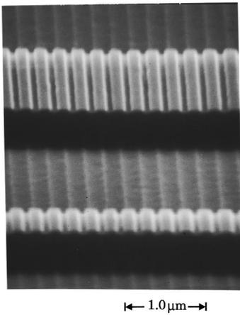
FIG. 2. SEM picture of the top-side views of the microfabricated strongly-guided AlGaAs Bragg filter waveguide.
