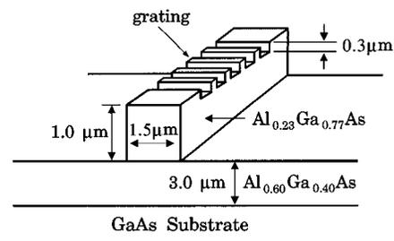
FIG. 1. AlGaAs Bragg filter waveguide structure.
