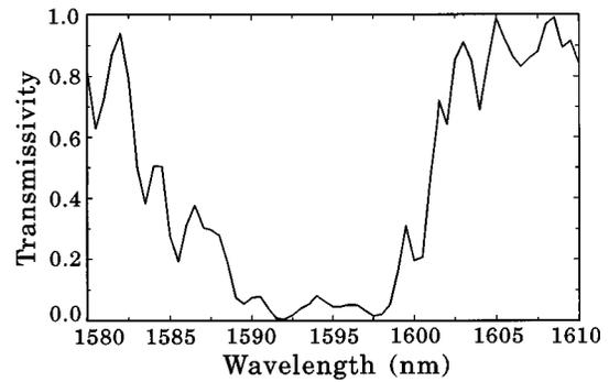
FIG. 4. Experimentally measured transmissivity spectrum of the AlGaAs Bragg filter with a FWHM bandwidth of about 15 nm.
