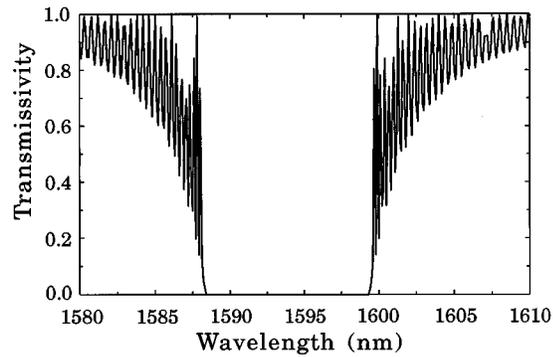
FIG. 5. Theoretically calculated transmissivity spectrum for a Bragg filter. The refractive indices used in the EIM calculations at  $\lambda=1.6 \mu\text{m}$  for the top, guiding, and cladding layers were  $n_t=1.0$ ,  $n_g=3.26214$ , and  $n_c=3.08689$ , respectively.
