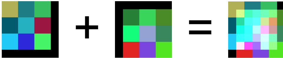
Figure 1: Overlapping sub-frames of pixels that are shifted a fraction of the pixel pitch, as in [13].
