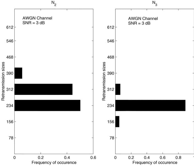
Fig. 5. Example of sizes  $N_2$  and  $N_3$  picked by the multitarget RBHARQ scheme in an AWGN channel, SNR = 3 dB.
