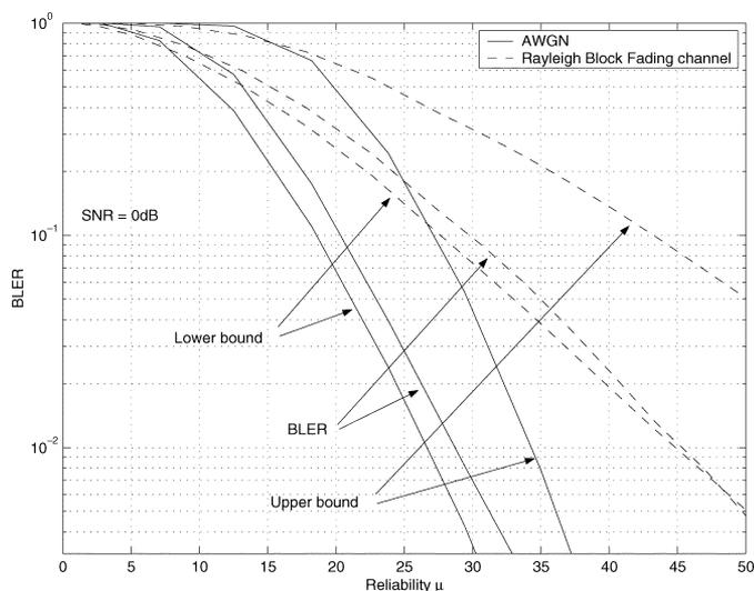
Fig. 9. Comparison of simulated  $F(\cdot)$  with the upper and lower bounds in (14).
