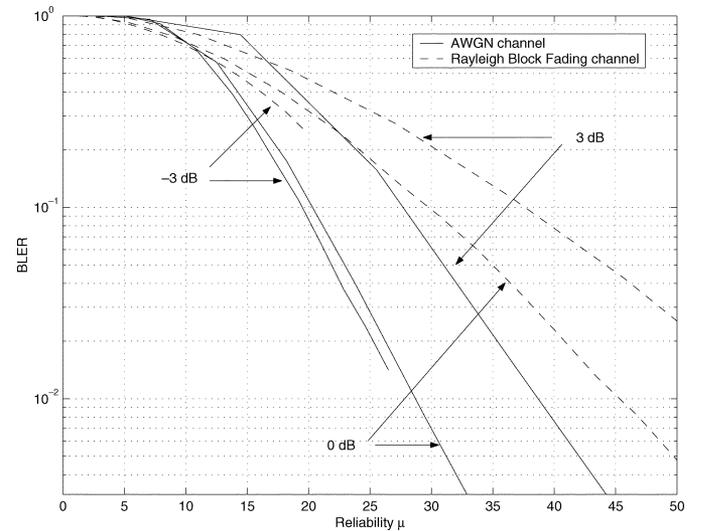
Fig. 2. Reliability to BLER mappings in AWGN and Rayleigh block fading channel models.
