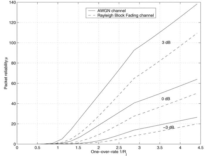
Fig. 1. Code rate to reliability mappings in AWGN and Rayleigh block fading channel models.
