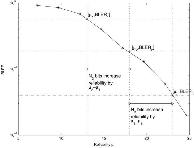
Fig. 3. Example of the the reliability to BLER mapping  $F(\cdot)$ .
