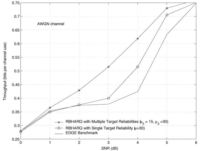
Fig. 4. Performance comparison in AWGN channel.
