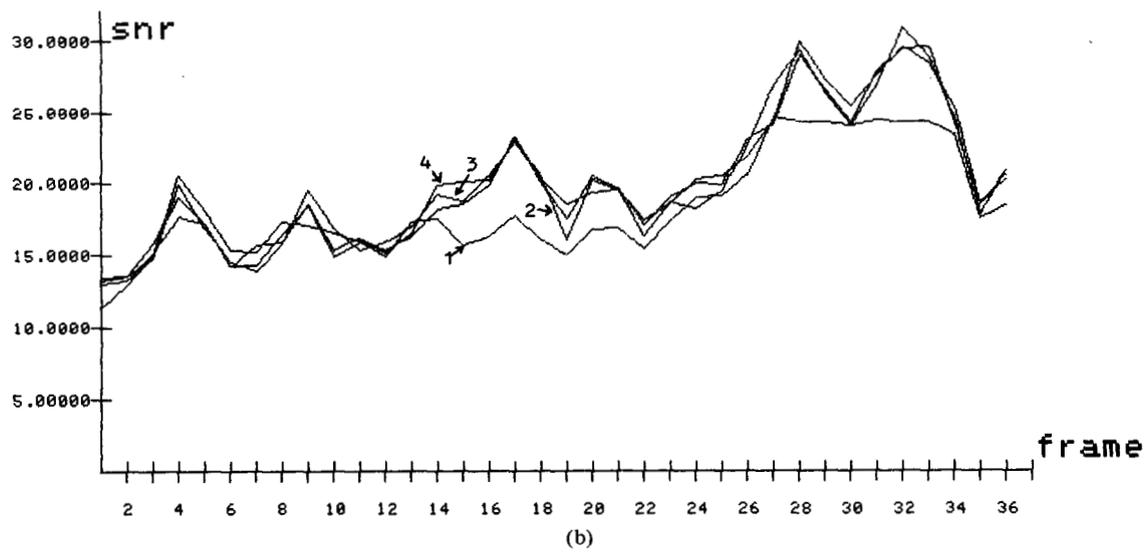
Fig. 5. (a) SNR obtained from using (curve 1) an LS lattice predictor and (curve 2) an LS lattice predictor plus pitch predictor for vowel sounds. (b) SNR obtained from using (curve 1) a fixed predictor, (curve 2) an LMS transversal predictor, (curve 3) an LMS lattice predictor, and (curve 4) an LS lattice predictor for vowel sounds.
