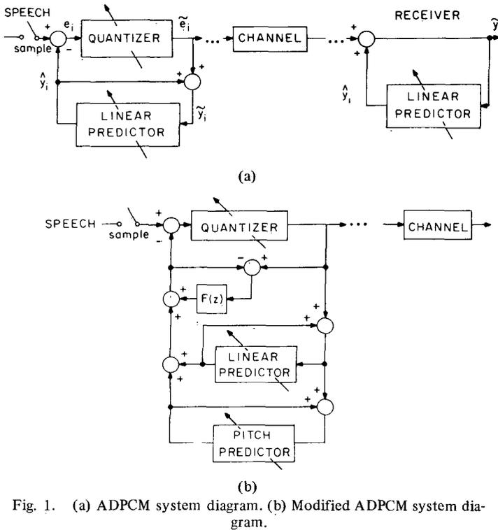
Fig. 1. (a) ADPCM system diagram. (b) Modified ADPCM system diagram.
