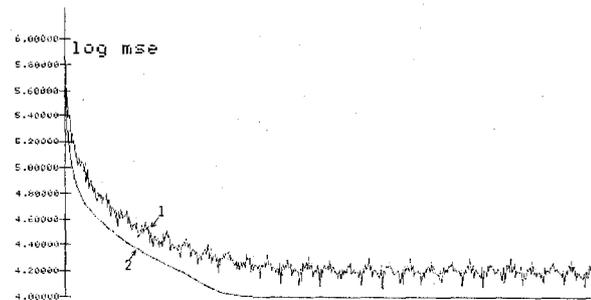
Fig. 5. Output MSE of a tenth-order lattice normalized gradient algorithm by (Curve 1) simulation and (Curve 2) from the model in Section IV.
