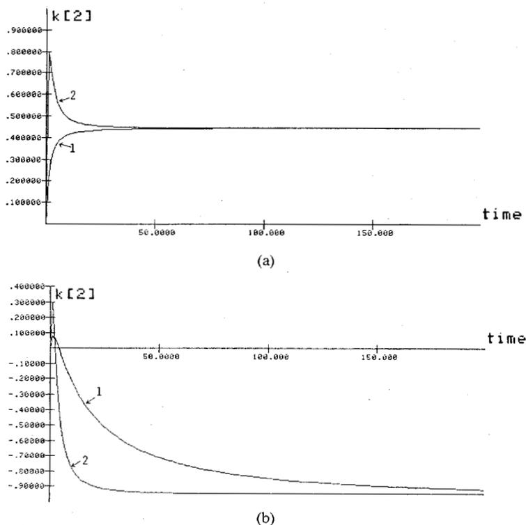
Fig. 6. Mean value trajectories (Curve 1) of the second PARCOR coefficient in a two-stage adaptive lattice (given by the model in Section IV) using different input statistics. Curve 2 shows the trajectory of  $k_{2,\text{opt}}(i)$ . Fig. 6(b) represents a "fast mode" of the filter, Fig. 6(b) represents a "slow mode."
