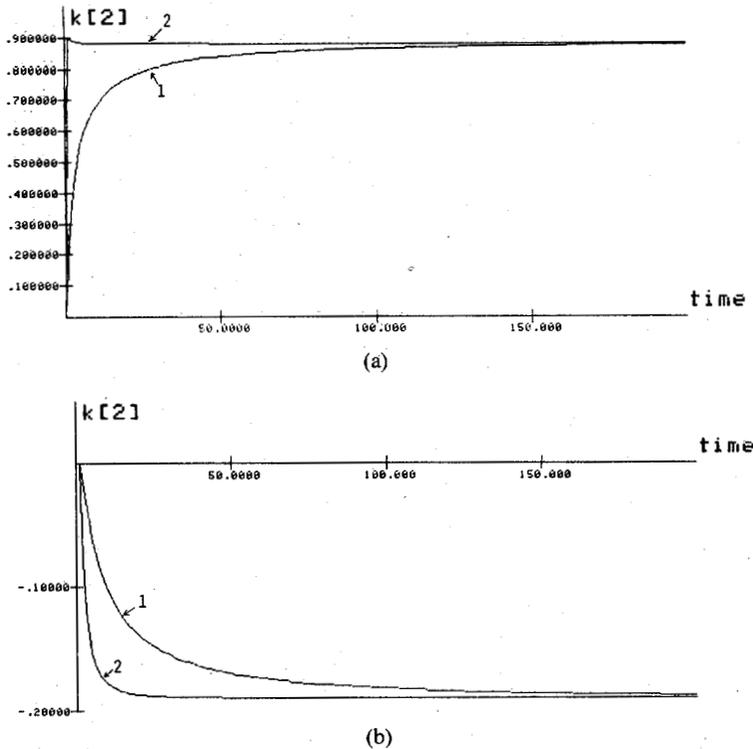
Fig. 7. Trajectories of (Curve 1)  $E[k_2(i)]$  and (Curve 2)  $k_{2,\text{opt}}(i)$  for a two-stage adaptive lattice using different input statistics. The value of  $R_1$  used in this case is significantly less than that used to generate the curves in Fig. 6.
