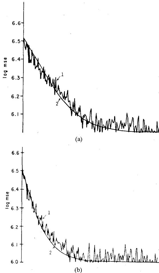
Fig. 8. Output MSE curves by (Curve 1) simulation and (Curve 2) from the model in Section IV for (a) a two-stage adaptive lattice, and (b) a two-stage adaptive transversal filter using equivalent initial conditions and input statistics.
