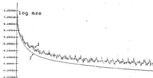
Fig. 4. Output MSE of a tenth-order lattice unnormalized gradient algorithm by (Curve 1) simulation and (Curve 2) from the model in Section IV.
