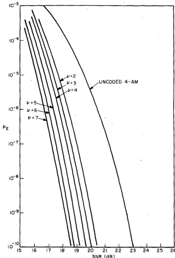
Fig. 4.  $P_E$  bound versus SNR for best 8-AM codes.
