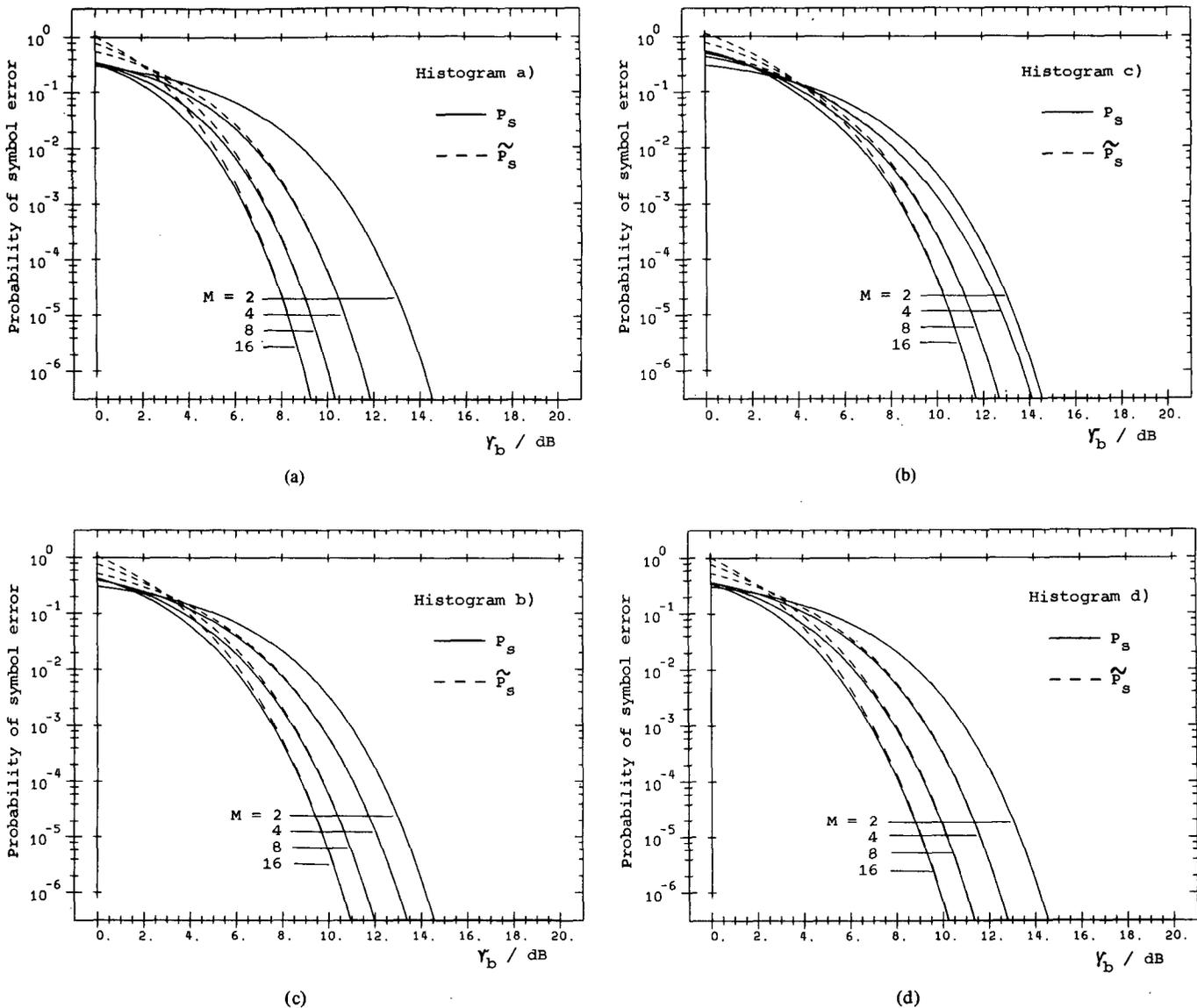
Fig. 3. Probability of error versus signal-to-noise ratio per information bit corresponding to the situation of interference as shown in Fig. 2(a)-(d).
