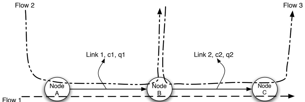
Fig. 1. Three flow, two link bottlenecked network example. Used to illustrate lack of convergence of bottlenecked conflicts despite the convergence of max-min fair solutions proved in Corollary 1. Also demonstrates the asymmetry in max-min fair solutions that is induced by lossy links.
