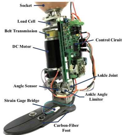
Fig. 1. The prototype of the proposed prosthesis PKU-RoboTPro-II.
