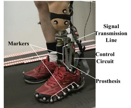
Fig. 4. Walking test experiment.
