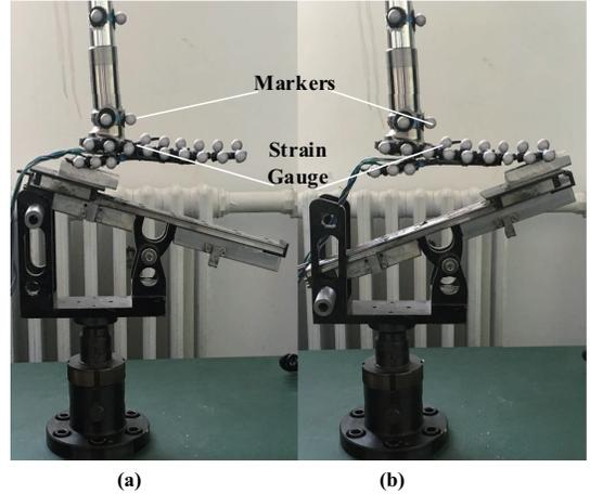
Fig. 3. The experiment on the relation between joint angle and strain gauge.
