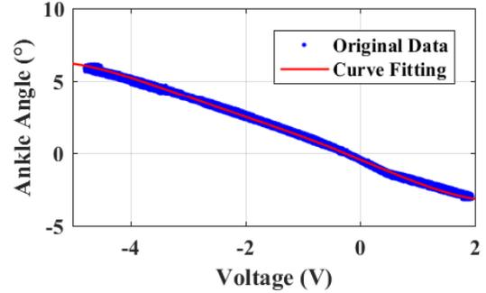
Fig. 5. Curve Fitting. The blue points refer to the original data. The red line refers to the curve fitting based on Fourier function.  $0^{\circ}$  indicates that the plane where the shank lies is perpendicular to the plane of the carbon-fiber foot plate. The positive angle represents the dorsiflexion and the negative angle represents the plantar flexion.
