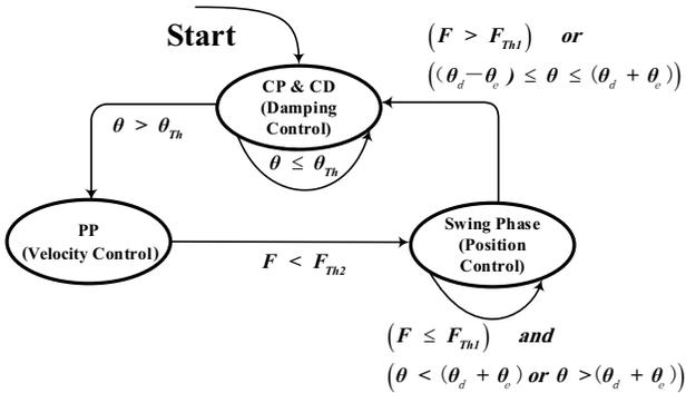
Fig. 2. Finite-state machine control diagram.  $F_{Threshold1}$  represents the gravitational pressure threshold at the instant of heel strike.  $F_{Threshold2}$  represents the gravitational pressure threshold while toe-off.  $\theta_{Threshold}$  represents a minimum angle to detect the beginning of push-off.  $\theta_e$  represents the allowable angle of error.  $\theta$  represents the ankle joint angle.
