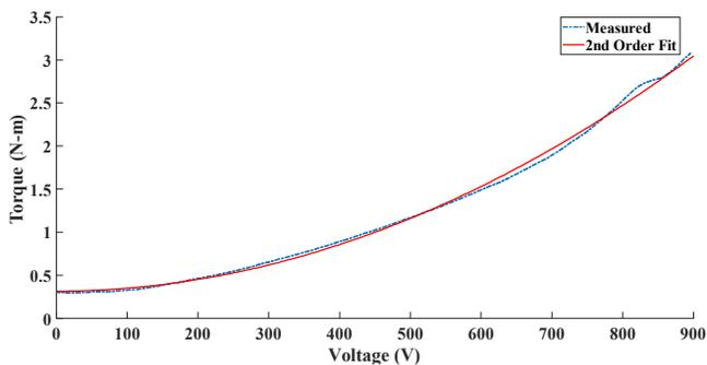
Fig. 2. Second order regression of the ER brake’s measured torque versus voltage.
