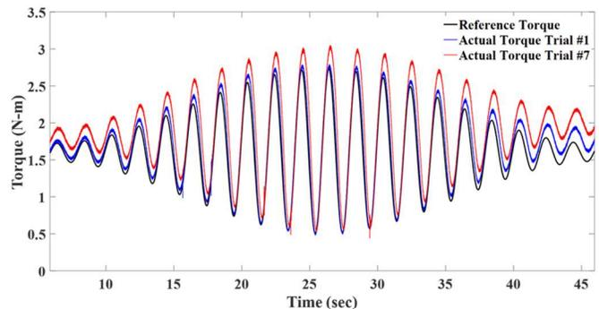
Fig. 3. Actual torques signals compared with a reference torque trajectory. The carrier wave was a 500 mHz sine wave with a 1.25 Vpp amplitude and 0.8 V offset. A 25 mHz amplitude modulation with 80% depth was applied to the reference trajectory.
