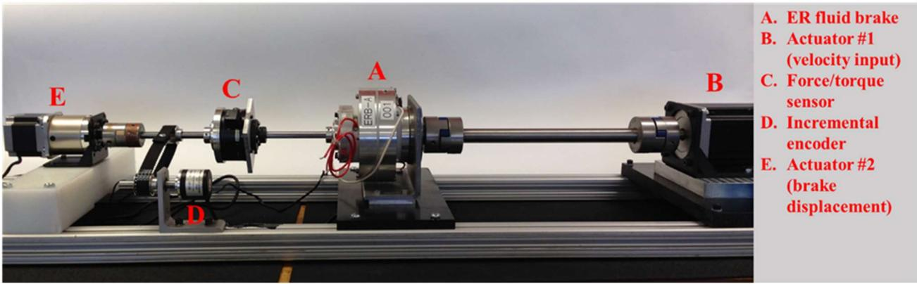
Fig. 1. Experimental setup used during the variable impedance study. One stepper motor provided a velocity source to shear the fluid internal to the brake while a second stepper motor displaced the body of the brake.
