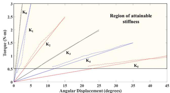
Fig. 5. Implementation of a virtual spring. The solid lines show the desired linear spring constants  $K_n$ .
