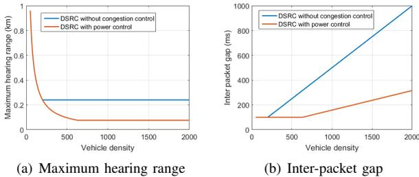
Fig. 9: Comparison for DSRC with and without power control.
