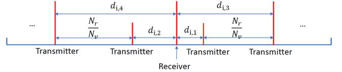
Fig. 2: Illustration of distances with multiple interferers.
