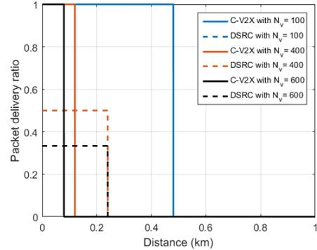
Fig. 6: Packet delivery ratio versus distance between receiving and transmitting vehicles under idealized scheduling for both C-V2X and DSRC.
