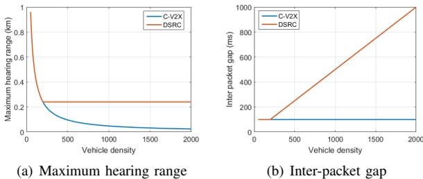
Fig. 7: Comparison between C-V2X and DSRC.
