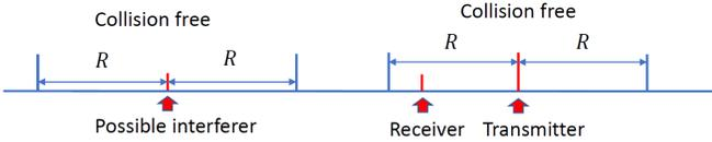
Fig. 5: Illustration of interference in DSRC.
