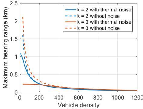
Fig. 3: Impact of noise and path loss factor on maximum hearing range.
