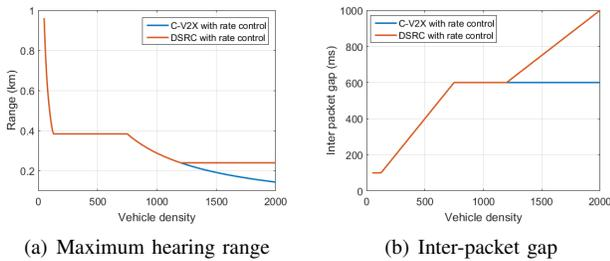
Fig. 8: Comparison between C-V2X and DSRC with rate control.
