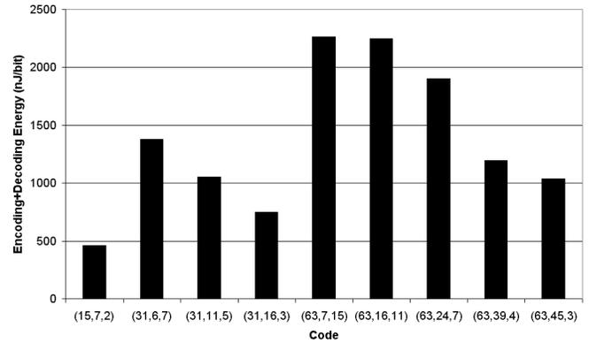
Fig. 13. Total energy consumption for encoding and decoding using BCH codes.
