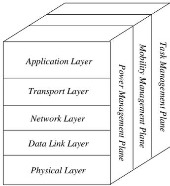
Fig. 3. The sensor networks protocol stack.
