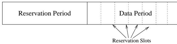
Fig. 9. General frame structure for TDMA-based MAC protocols.
