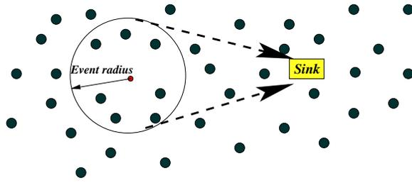
Fig. 4. Typical sensor network topology with event and sink. The sink is only interested in collective information of sensor nodes within the event radius and not in their individual data.
