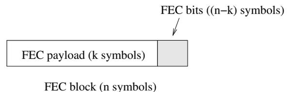
Fig. 11. An illustration of forward error correction (FEC) in WSN.
