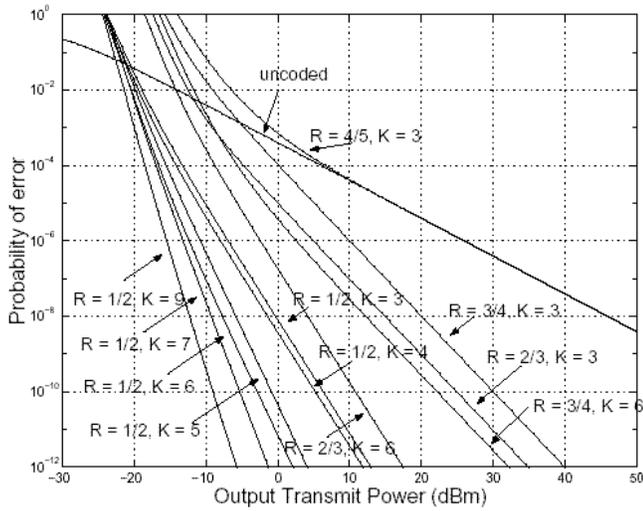
Fig. 12. Probability of error versus transmission power for different convolutional codes.
