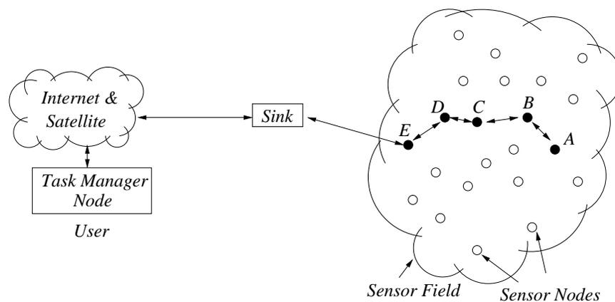
Fig. 2. Sensor nodes scattered in a sensor field.
