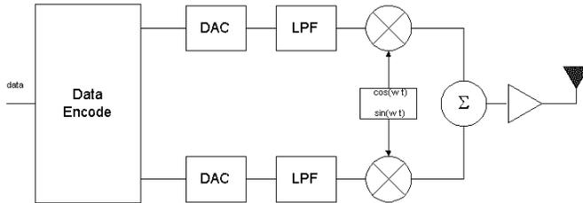
Fig. 16.  $M$ -ary Modulation Block.
