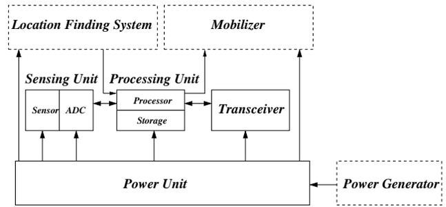
Fig. 1. The components of a sensor node.
