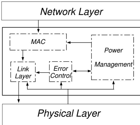
Fig. 10. An overview of data link layer providing reliability in WSN [221].
