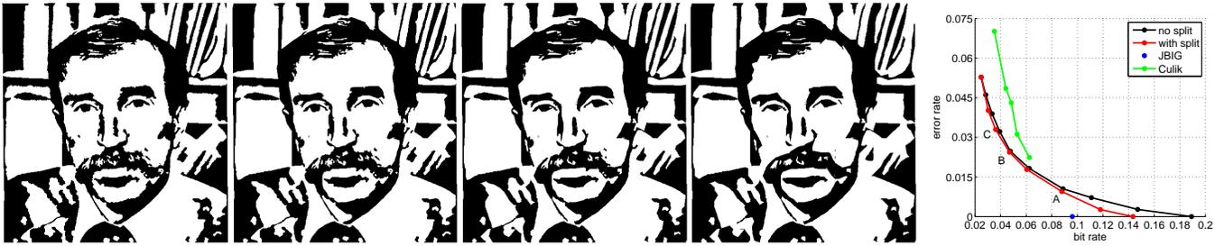
Fig. 4. Hierarchical coding examples: Original, .09 bpp (A), .05 bpp (B), .04 bpp (C) (left to right), rate-distortion curves
