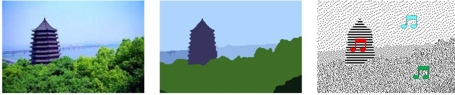
Fig. 2. Visual to acoustic-tactile mapping. (left) Original color image; (middle) segmentation; (right) acoustic-tactile display.
