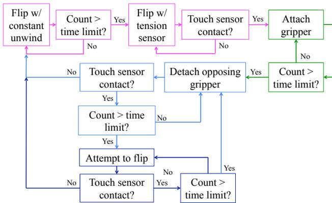
Fig. 5. Flow Diagram for Control 1 (first simple control algorithm). Each color represents a different state.
