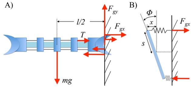
Fig. 4. a) Free body diagram of the robot vertical climbing in its extended position. The motor winding the cable must balance the moment arm of the robot as well as the resistance to bending of the flexible joints. Similarly the gripper must be able to hold the moment arm of the robot. b) Model of the corkscrew gripper as spring point forces
