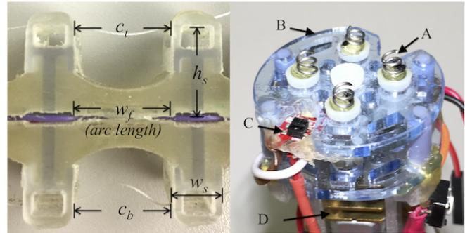
Fig. 3. Left: Close up of a body segment. The flexible segment is concave to encourage bending at the middle. Right: Close up of corkscrew gripper: A) Corkscrews mounted on Lego gears B) Acrylic housing C) IR reflectance sensor D) Gripper motor
