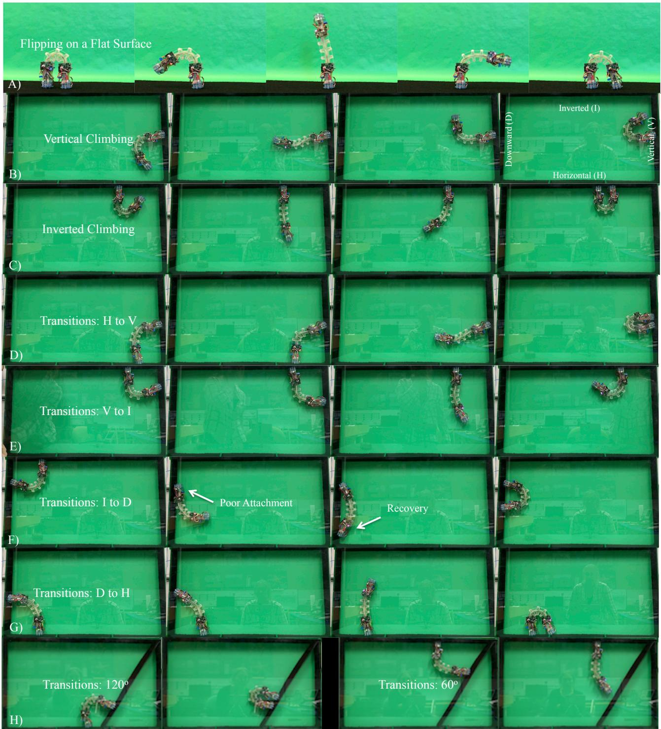
Fig. 7. Video stills of Flippy robot on a flat, unconstrained track (A) and 2D constrained track (B-H). B) Horizontal to Vertical transition, C) Vertical climbing, D) Vertical to Inverted transition, E) Inverted climbing, F) Inverted to Downward transition, G) Downward to Horizontal transition, H) Climbing and transitioning over approximately 120° and 60° angled surfaces
