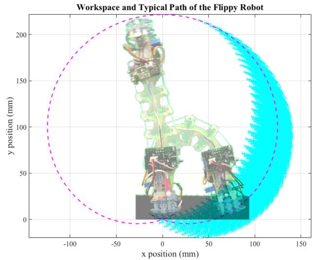
Fig. 2. Flipping trajectory of the robot. The dotted line shows a typical flip, assuming equal bending in all sections. The blue markers show the workspace of the robot.
