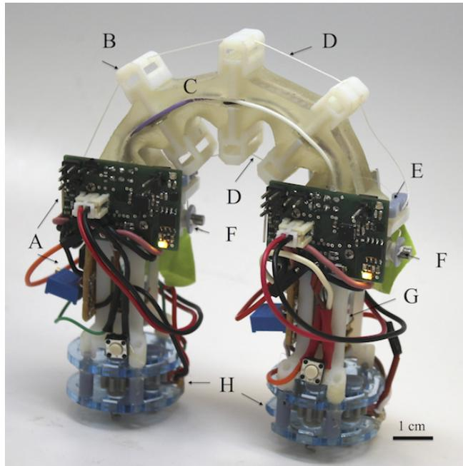
Fig. 1. Flippy robot. A) Printed circuit board and additional board for IR sensor circuit B) Stiff body part C) Flexible body part with embedded wire to connect between boards D) Cable E) Tension sensor: a pin joint link which pushes a switch on the PCB when the cable is in tension F) Winding spool and motor G) Gripper motor H) Corkscrew gripper with housing
