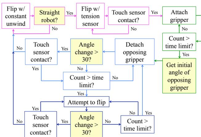
Fig. 6. Flow Diagram for Control 2 (control algorithm with IMU sensing). Changes from Control 1 are highlighted.
