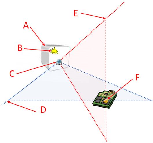
Fig 2: (A) Vive Lighthouse. (B) Omnidirectional IR Flash. (C) High speed mirror and laser beam. (D) Y axis value. (E) X axis value. (F) Vive sensor.
