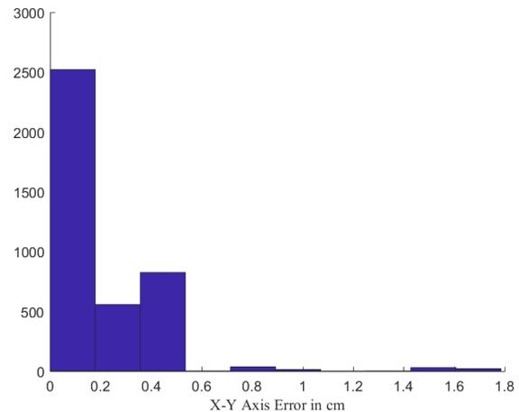
Fig. 6. X&Y axis error histogram in cm. Computed from 2000 measurements, 50% at 100cm and 50% at 75cm from the lighthouse.
