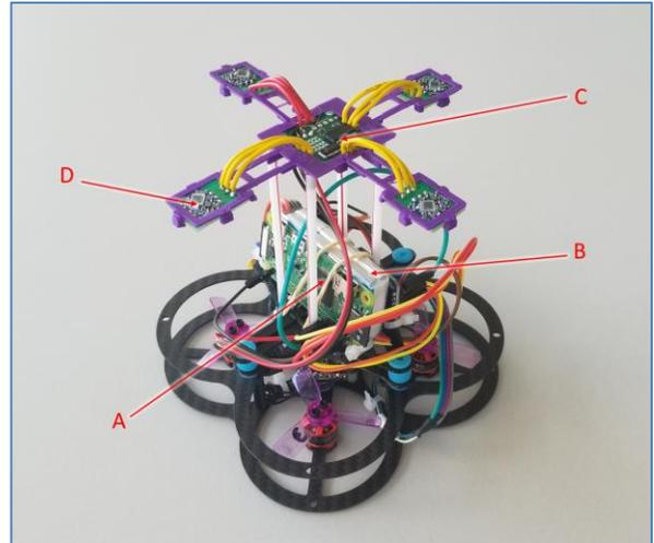
Fig. 1. Quadcopter drone with the Raspberry PI Zero W board (A), a 500mAh battery (B) and the high resolution 3D positioning device (C) showing the set of four Vive™ sensors (D).
