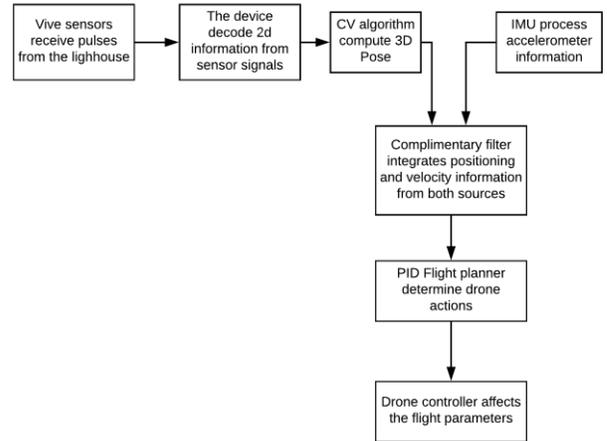
Fig. 3. Data gathering and processing flowchart.
