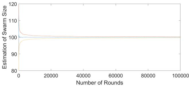
Fig. 3: The average, and 1 standard deviations above and below average of 1000 experiments with 100 simulated robots as increasing number of rounds are included in the size estimate.
