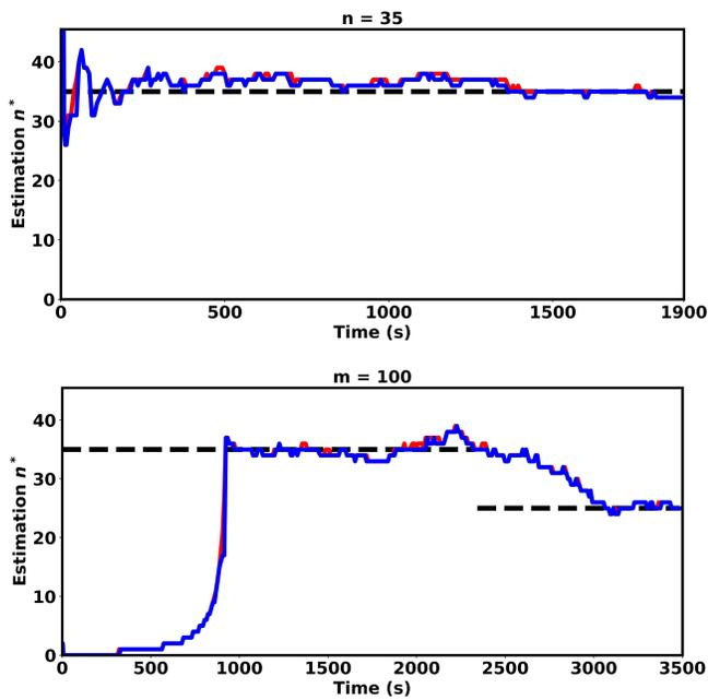
Fig. 7: The results from physical experiments. The black dotted line is the actual swarm size  $n$ , the red and blue solid lines are largest and smallest estimation amongst the swarm, respectively.
