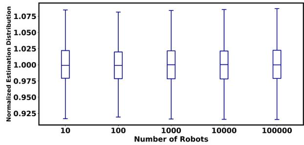
Fig. 1: The distribution of estimates for the number of robots for varying swarm size. The distribution is normalized by the true number of robots. Each boxplot represents the distribution of 2000 experiments in which the swarm used 1000 rounds to estimate the number of robots.
