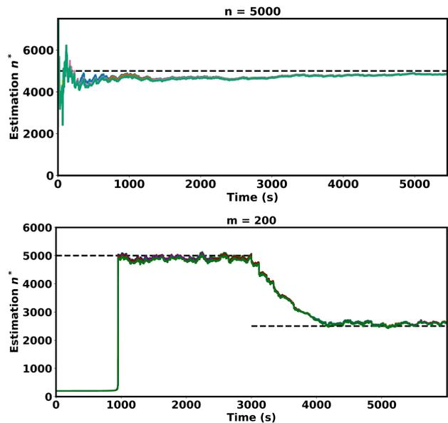
Fig. 6: The experiments to demonstrate the algorithm’s performance on a swarm of 5000 agents. The black dotted line is the actual swarm size  $n$  and the solid colored lines are agents’ estimations over time. The different colors indicates the results from different agents, plots are overlapping as many have similar estimates.
