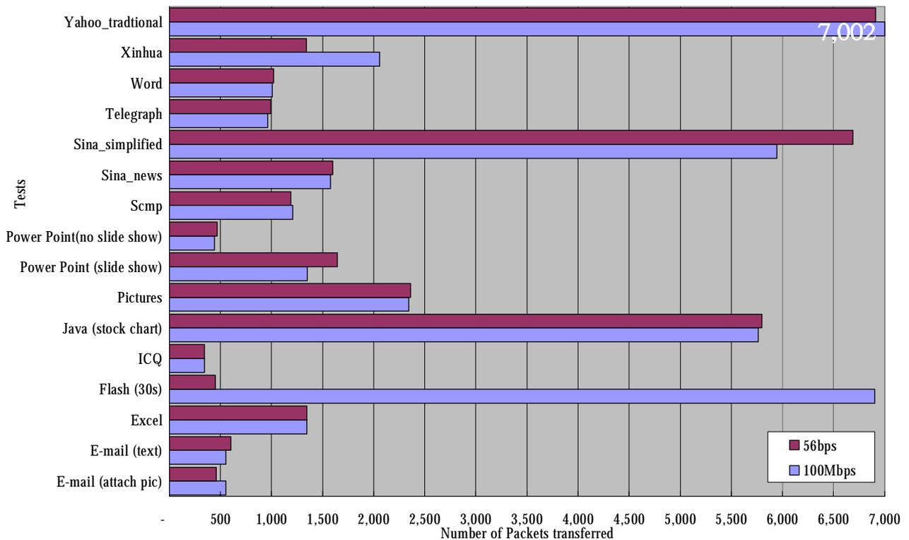
Fig. 24 Time for completion in different tests (100Mbps, 56kbps)
