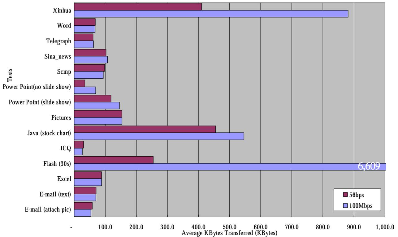
Fig. 23 Number of packets transferred in different tests (100Mbps, 56kbps)
