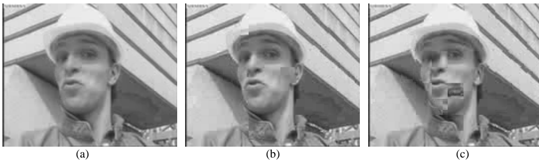
Fig. 1. (a) Expected reconstructed frame averaged over all possible loss simulations. (b and c) Reconstructed frames for two different channel loss realizations.
