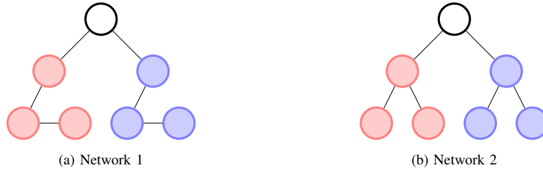
Fig. 2. Two radial networks that have different local topologies but the same socially optimal and equilibrium supply profiles. The nodes with the same color are homogeneous, while the nodes with different colors can be different.
