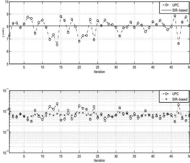
Fig. 3. User 1 output SIR and BER for the UPC algorithm and SIR-based algorithm with the MMSE receiver ( $N = 32$  and  $K = 8$ ).
