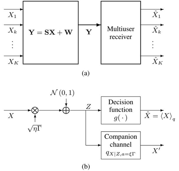
Fig. 1. (a) The DS-CDMA system with multiuser detection. (b) The equivalent scalar Gaussian channel for user  $k$  and the companion channel.
