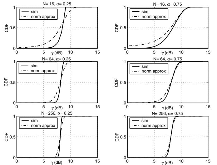
Fig. 5. CDFs of  $\gamma$  for the MMSE receiver.
