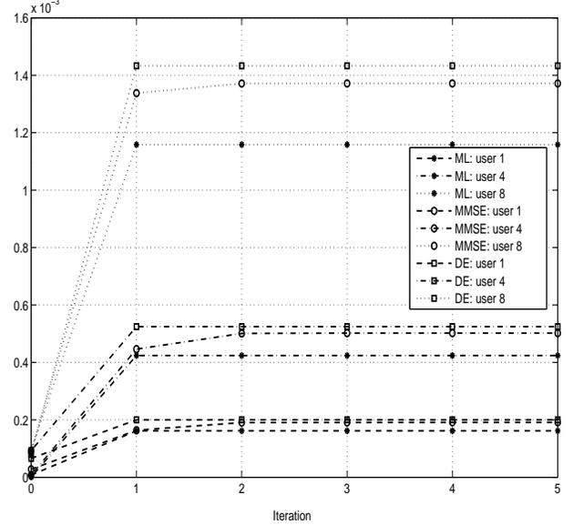
Fig. 2. Transmit powers for the ML, MMSE, and decorrelator, using the UPC algorithm ( $N = 32$  and  $K = 8$ ).
