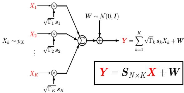
Fig. 1. System Model for Uplink CDMA
