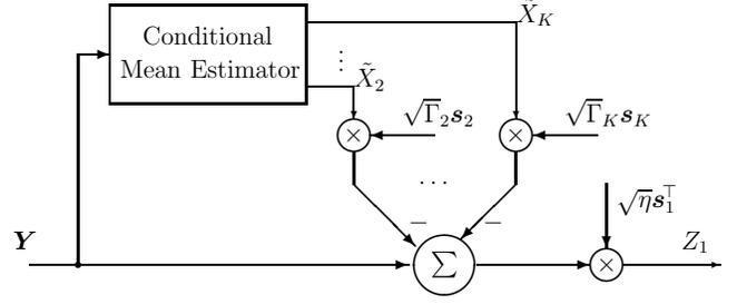
Figure 3: A canonical interference canceller equivalent to the conditional mean estimator.
