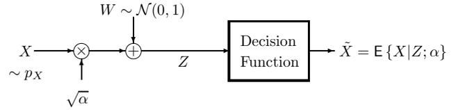
Figure 2: Equivalent single-user channel.
