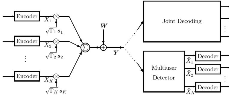
Figure 1: System model of CDMA with joint or separate decoding.
