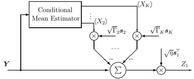
Figure 3: A canonical interference canceler equivalent to the conditional mean estimator.
