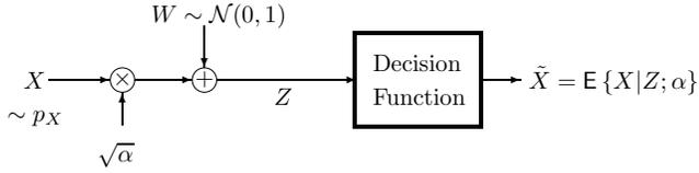
Figure 2: Equivalent single-user channel.
