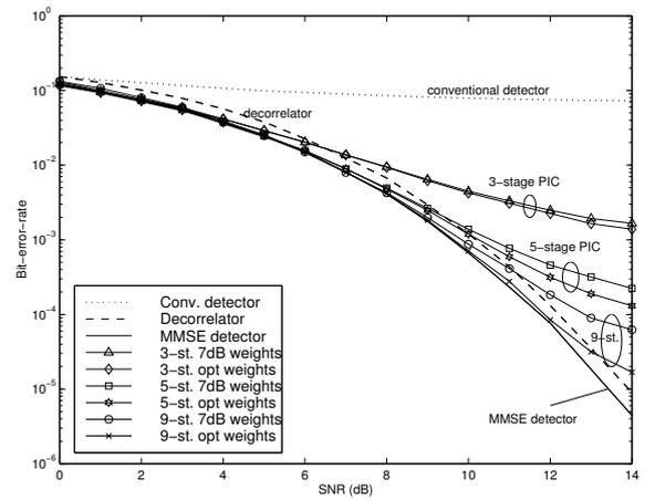
Fig. 5. BER performance and sensitivity versus SNR using long codes. Weights optimised for 7 dB are used for 0-14 dB, in comparison to when the weights are optimised for the actual SNR. Here,  $N=31$ ,  $K=15$  and  $\beta_k=\beta$  (perfect power control) is assumed.
