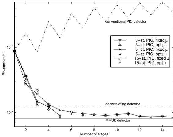
Fig. 3. BER performance as a function of the number of stages. Both the cases of a fixed set of weights as well as optimal weights for each symbol interval are included. Here,  $\text{SNR}=7$  dB,  $N=31$  and  $K=15$ .
