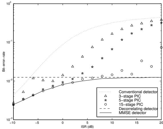
Fig. 4. Near-far ability of the weighted linear PIC for a long-code system.  $N=31$ ,  $K=15$  and the SNR for user 1 is  $\beta_1=7$  dB while for all other users  $\beta_k=7+\text{ISR}$  dB. The performance of user 1 is shown.
