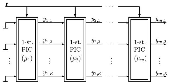
Fig. 1. General structure for a  $K$ -user,  $m$ -stage PIC.
