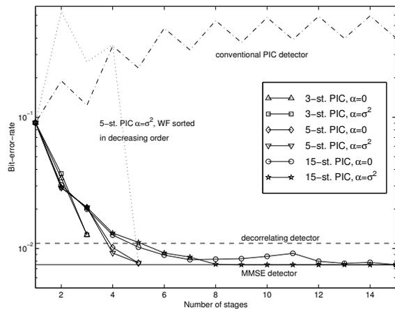
Fig. 3. Stage-by-stage performance of PIC detector with optimal weighting factors (WF) using short codes.
