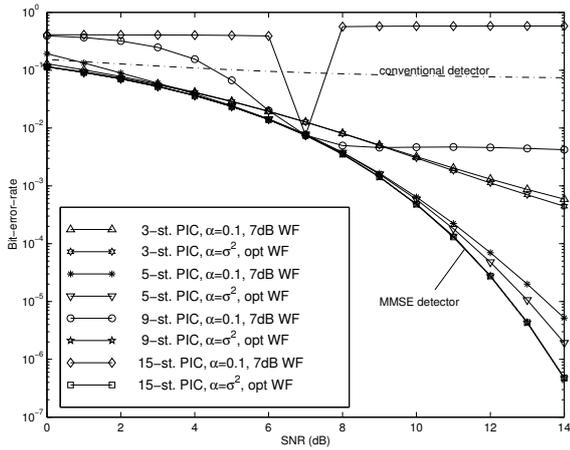
Fig. 5. BER performance and sensitivity vs. SNR using short codes. Weighting factors (WF) optimised for 7 dB and  $\alpha = 0.0998$  (simplified to  $\alpha = 0.1$  in the legend) are used for 0-14 dB, in comparison to when the weights are optimised for each working SNR and corresponding  $\alpha$ .
