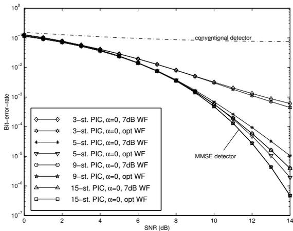
Fig. 6. BER performance and sensitivity vs. SNR using short codes. Weights (WF) for 7 dB are used for 0-14 dB, in comparison to when the weights are optimised for each working SNR.  $\alpha = 0$  is assumed in all cases.
