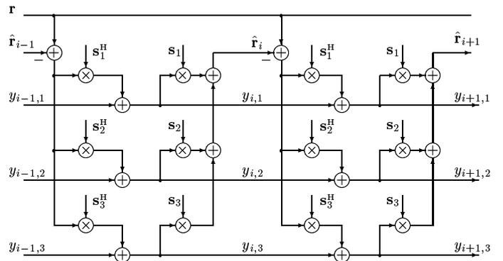
Fig. 1. The conventional PIC structure for a 3-user case. Stages  $i$  and  $(i+1)$  are shown. Assume that  $\hat{\mathbf{r}}_0 = \mathbf{0}$  and  $y_{0,k} = 0$  for all  $k$ 's.
