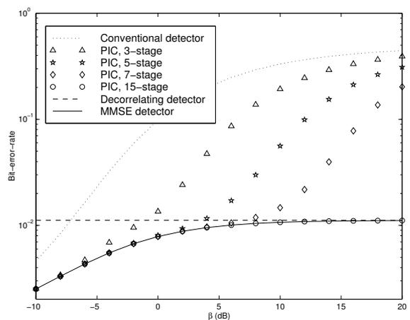
Fig. 4. Near-far ability of the weighted PIC using short codes.
