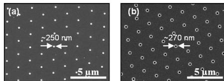
FIG. 5. SEM images: (a) photoresist nanopillar array with a different pitch size ( $\sim 2 \mu\text{m}$ ); (b) nanohole array perforated in titanium film with a different pitch size ( $\sim 2 \mu\text{m}$ ).
