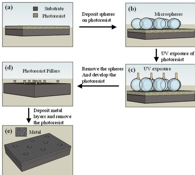
Fig. 1. Schematic illustration for forming perforated hole arrays in metal layer.
