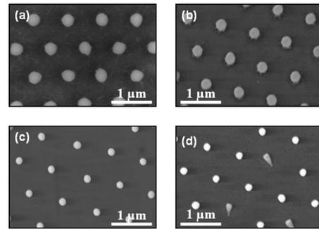
Fig. 3. SEM images of photoresist pillars with different development times of MIF-300: (a) underdeveloped photoresist, the development time is about 30 s; (b) the development time is about 40 s, there is still photoresist around the pillars; (c) the development time is about 50 s, perfectly nanopillars formed; (d) overdeveloped photoresist, the pillars began to fall down, the time is about 60 s.
