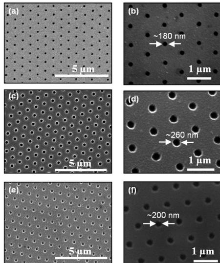
FIG. 4. SEM images: (a) gold hexagonally packed hole arrays; (b) enlarged view of (a); (c) aluminum hole array; (d) enlarged view of (c); (e) aluminum/aluminum oxide hole array; (f) the enlarged view of (e).
