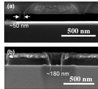
FIG. 6. SEM images: (a) cross-sectional view of holes in aluminum with a strong undercut sidewall, (b) cross-sectional view of holes in silicon dioxide/aluminum with vertical sidewall.
