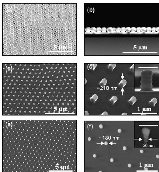
Fig. 2. SEM images: (a) hcp monolayer of spheres on top of photoresist; (b) cross-sectional view of (a); (c) nanopillar arrays of photoresist developed by ma-D 331S; (d) enlarged image of (c); (e) nanopillars of photoresist developed by MIF-300; (f) enlarged view of (e); insets of (d) and (f) show single pillars (the scales are both 400 nm).
