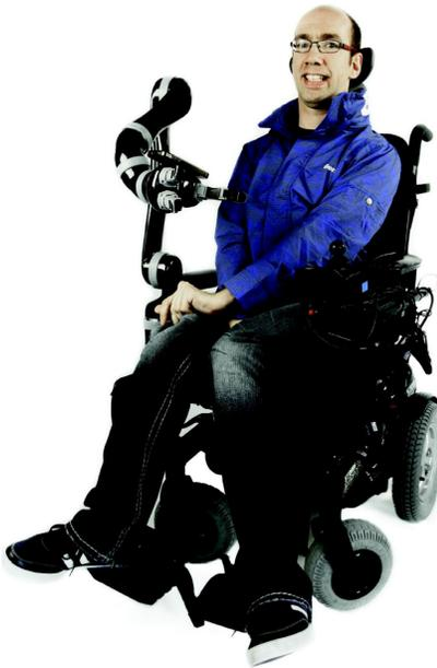
Figure 1. The MICO robotic arm on a power wheelchair with user. <http://www.kinovarobotics.com/>
