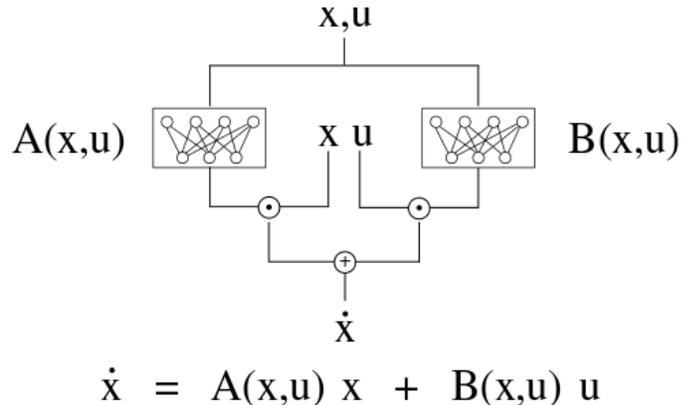
Fig. 1: Structured neural network architecture for model-based predictive control. The final layer of the  $A$ -subnet must be the same dimension as the state space, and the final layer of the  $B$ -subnet must be the same dimension as the control space. The network then computes a function of the form  $\dot{x} = A \cdot x + B \cdot u$ . This structure makes it easy to recover time-varying derivatives (i.e.,  $A, B$ ) for use in model predictive control algorithms.
