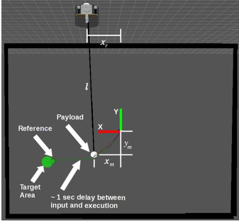
Fig. 1. Definition of the system configuration variables  $x_m$ ,  $y_m$ ,  $x_r$  and  $l$ . The delay between user input (green line) and execution (blue line) is approximately 1 second.
