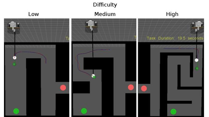
Fig. 2. Example maze environments for the simulated planar crane task, showing initial position (red circle), target position (green circle), current position of the user input (smaller green sphere), reference trajectory (blue line), executed trajectory (red line), suspended mass (white circle), and maze walls (black). A robotic winch (grey) manipulates the location and length of the string supporting the payload.
