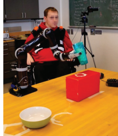
Fig. 5. An SCI user controlling the robot with the BMI during the experimental task.
